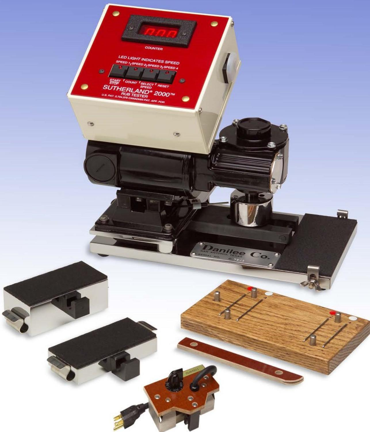
Illustrated is the 4-speed SUTHERLAND® 2000® Rub Tester showing the two-pound and four-pound weights to which test specimens are attached and the scoring device which are the standard equipment for the instrument. The receptacle is the same voltage as the instrument. 110 volts single phase is standard. 220 volts optional at extra cost.
