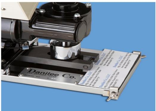
Step 5. Place your 2 5/8 inch by 6 inch (66 mm by 150 mm) printed stock test specimen on the base pad of the unit, printed side up. Attach the hold down brackets to secure the test specimen from movement.
