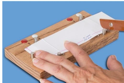
Step 8. To prepare samples for the 4-pound weight, The 2 inch by 7 inch (50 mm by 177 mm) strips are placed face up against the end pin of the scoring device (wooden block), on top of the wires (as shown), then 'scored' using the micarta scoring tool at the white dot positions. This will facilitate bending the strips to conform to the test weight.
