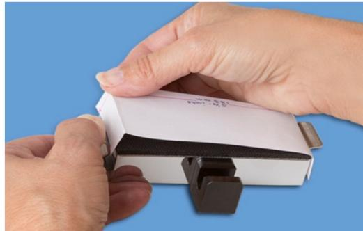
Step 4. Placing the strip on the 2-pound weight. The test strip should be placed under one clip with the scoring lined up with the edge of the weight. Smooth the test strip across the bottom of the weight and attach the other end under the opposite clip.
