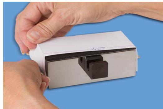
Step 9. Placing the strip on the 4-pound weight: the test strip should be placed under one clip with the scoring lined up with the edge of the weight. Smooth the test strip across the bottom of the weight against the pad and attach the other end under the opposite clip on the weight.
