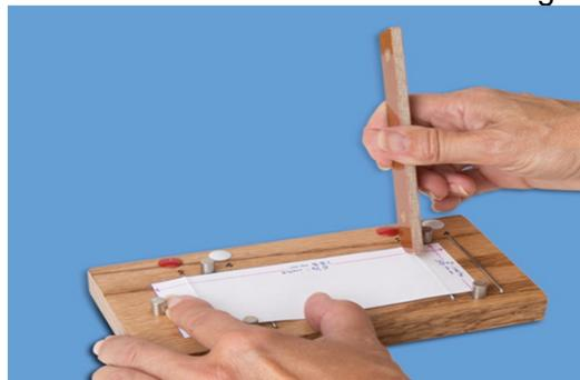
Step 2. To prepare samples for the 2-pound weight: The 2 inch by 5 ¼ inch (50 mm by 135 mm) strips are placed face up against the end pin of the scoring device (wooden block) and on top of the wires (as shown). Then “scored” using the micarta scoring tool at the red dot positions. This will facilitate bending the strip to conform to the test weight.
