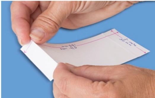
Step 3. Bend the test strip at the “scores”, this will help it to lie flat on the weight pad.
