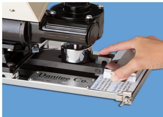
Step 6. Place the weight (with the receptor attached) on the arm of the unit by slipping the hook into the arm over the pin. The weight should lay flat on the test specimen. The machine should **NOT** be running.
