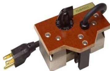
This heated weight provides a uniform test for evaluating the "hot abrasion" resistance of printed cartons, labels, etc. Where required, rub resistance specifications may now be based on number of strokes at a given temperature as well as pressure. (refer to "Notes on the SUTHERLAND® Heated Weight & Suggested Procedures...")
